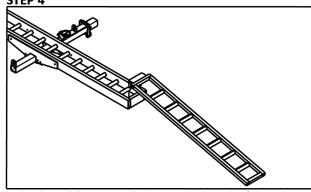
To load your bike, mount the ramp onto the side of the rail as shown.
