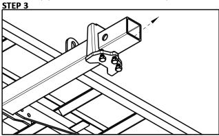
Insert the Anti-tilt bracket onto the Main Tube and insert the carrier into your hitch receiver. After securing the carrier with your hitch pin, push the Anti-tilt bracket against your hitch collar and tighten the 3/8" bolts. Loosely tighten the center bolt first to ensure that if fits just behind the lip of the hitch collar before tightening the side bolts. This prevents the bracket from slipping on rounded hitch collars. After tightening the sides, finish tightening the center bolt.
