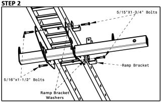
Secure the Rail and the Ramp Bracket to the Main Tube using the (2) 5/16" x 1-1/2" Bolts and (2) 5/16" x 1-3/4" Bolts where shown in the figure above. Place one of the (2) Ramp Bracket Washers between each Ramp Bracket and Rail Bracket. Tighten all Bolts with Lock Nuts (including those from Step 1). The Side of the Rail with the empty slot will be where the front tire of your bike sits.
