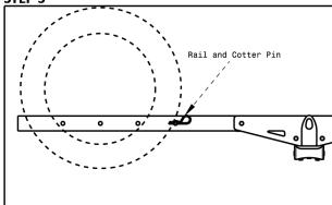
Insert the Rail Pin into the appropriate hole for your specific tire size, such that your bike's tire is supported and resting on the rail. Lock the Rail Pin with the Cotter Pin.
