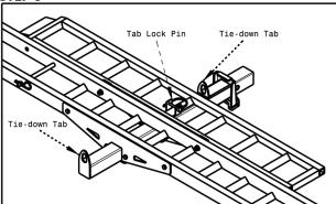
Secure the Ramp on the Main Tube using the Tab Lock Pin when it is not being used. Secure your bike with straps (not provided) using the Tie-down Tabs as shown.
