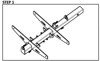
Mount the Rail Brackets to the Main Tube by using the 5/16" x 3/4" Bolts and Lock Nuts. Do not tighten, leave the bolts loose for now.
